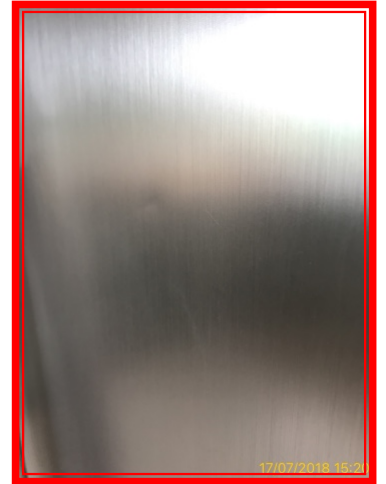
5.18.1 Some small dents to front of fridge .
